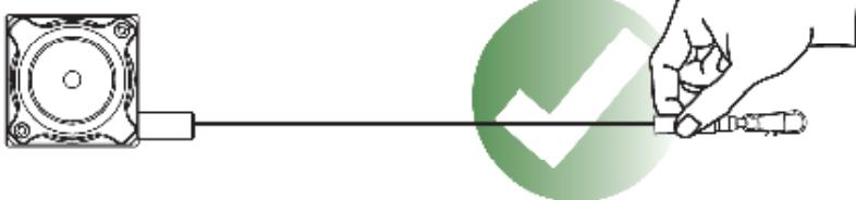
The wire must be extracted from the sensor vertically.
